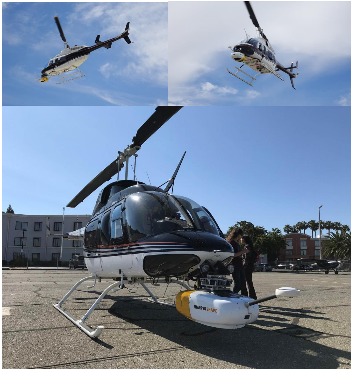
Caption: A Bell Long Ranger and/or a Bell 407 helicopter equipped with the LiDAR and high-resolution imaging will survey electrical equipment throughout Central and Northern California to identify potential wildfire risks.
